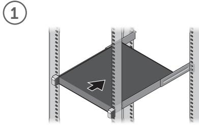
Install the system into a rack.
