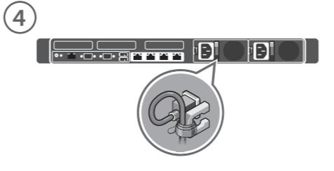
Loop and secure the power cable using the retention clip.
